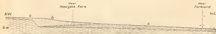
c. Buried cliff. b. Brickearth, s. Shingle of Raised Beach. b.m. Bembridge Marls, in which the raised-beach platform is cut.
